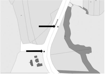
Figure 4 – Fire hydrant location
