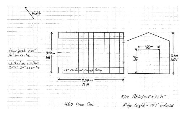
Figure 3 – Side view of proposed shed
