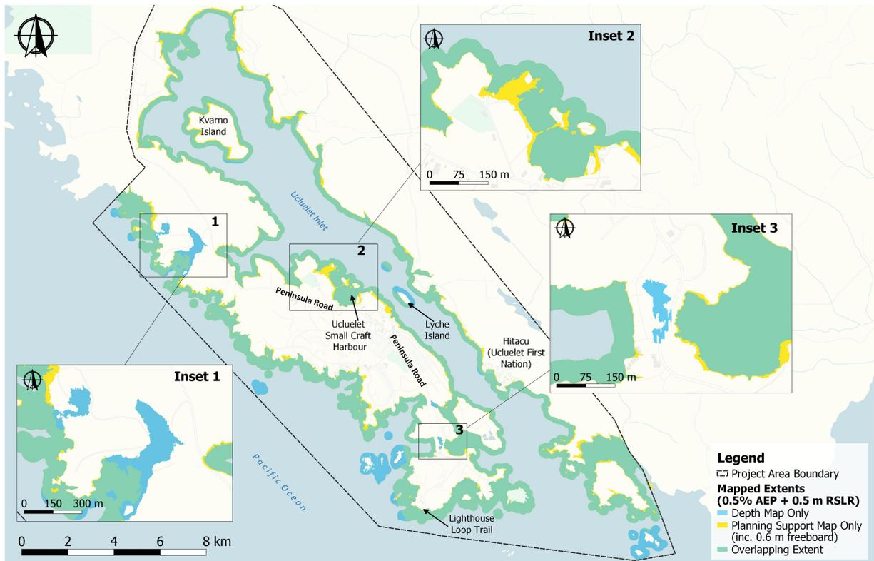
Figure 4: Map showing differences in the planning support and depth map extents for the 0.5% AEP + 0.5 m RSLR scenario.
