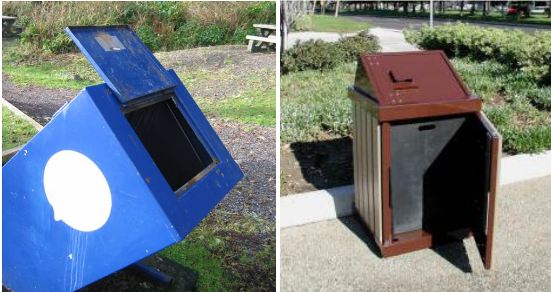
Figure 3. One of the receptacles at Big Beach (left) purchased in mid 1980s has rusted and lost its latch, rendering it no longer “wildlife resistant”. The plan is to replace this and other municipal receptacles in 2006-07 with “animal-proof” receptacles like the one shown on the right.
