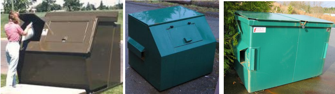
Figure 1. Garbage dumpster with a snug self-latching door (centre) is more “bear-resistant” than dumpsters with overhanging lids that need to be locked with a chain (right). The Haul-All dumpster on the left is the style preferred by National Parks and BC provincial parks because it is “animal-proof”. Bears cannot open the top or back because there is no edge to grip, unlike the dumpsters shown centre and right.
